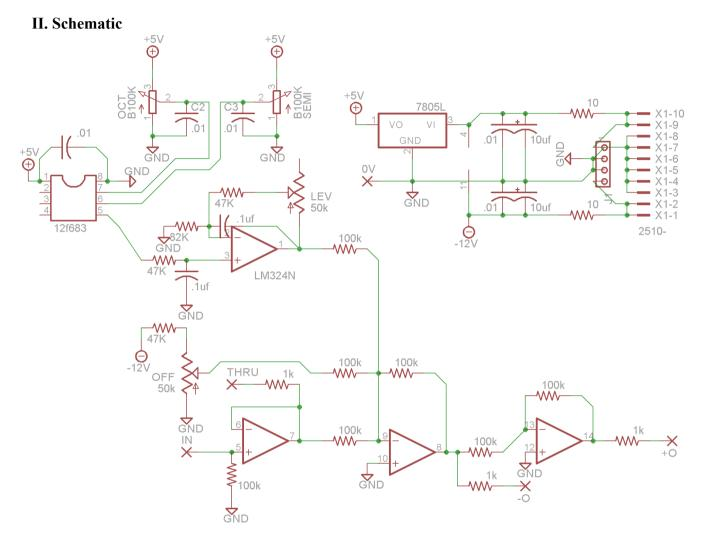
Above is the schematic for this module. In the upper left is the 12F683 PIC microcontroller, powered by +5V with a .01uf capacitor filtering it's power supply pin. Pins 6 and 7 each connect to the wiper of a 100K potentiometer wired as a variable voltage source ranging from 0 to +5V, with .01uf capacitors filtering any noise from the pots.
