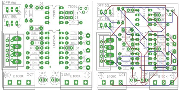
Above are images of the circuit board, with and withou traces shown. The ground fill plane is not shown on the image with traces. The PCB measures 48mm x 45mm with the pots spaced 30.48mm apart.
