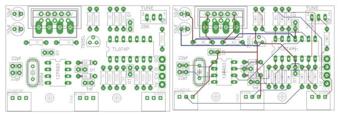
Above are renderings of the PCB with and without traces shown. The ground plane isn't shown, so some empty pads are connecting to ground. The PCB is 62mm x40mm. The pots are spaced 25.4mm apart and the mounting holes are 25.4mm apart from each other.
