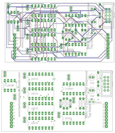
Below are renderings of the panel PCB with and without traces:
