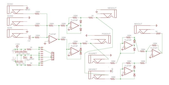
Above is the schematic for this module. Starting in the upper left are the DC and AC input jacks. All of these are in series with 100K resistors that meet at the negative input of an op-amp, with the AC jack also in series with a .1uf capacitor. The op-amp mixes and inverts these voltages and then sends them to a pair of inverting half-wave converters.
