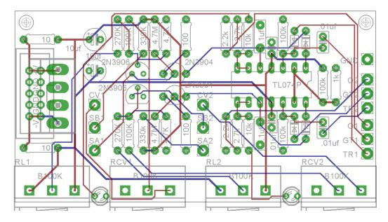
WIRING, repeat for each channel : SA – Wire to the bottom lug of the Slow Toggle SB – Wire to the middle lug of the Slow toggle. CV – Wire to tip of the CV jack. TR – Wire to the tip of the Trigger In Jack GT – Wire to the tip of the Gate In Jack O – Wire to the tip of the output Jack GND – Wire to the sleeve of any jack.
