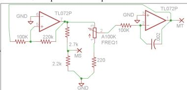
square wave output marked "MS" through a voltage divider (the schmitt trigger outputs  $\pm$ 12V, these resistors attenuate it down to  $\pm$ 2V). It then goes through a pot resisting the flow of current into the integrator, the 220 ohm resistor between the pot and ground sets the minimum frequency.
