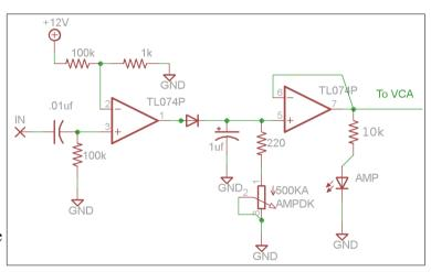
When the output goes high, current flows through this diode quickly charging the 1uf capacitor. The 220 ohm resistor and 500KA pot in parallel with the capacitor provide a path for the capacitor to discharge the voltage. The higher the resistance, the more slowly the capacitor discharge.
