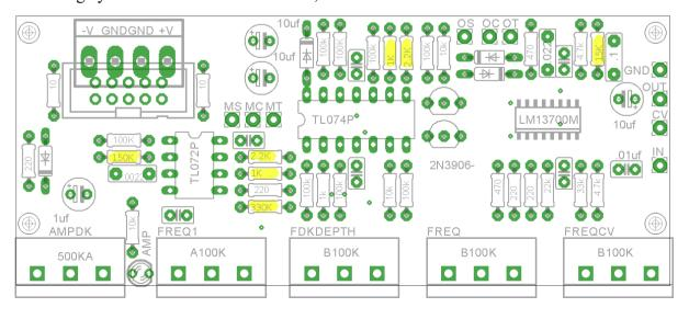
Below is an image of the PCB with the traces shown, to aid in troubleshooting. The ground fill plane is not shown.
