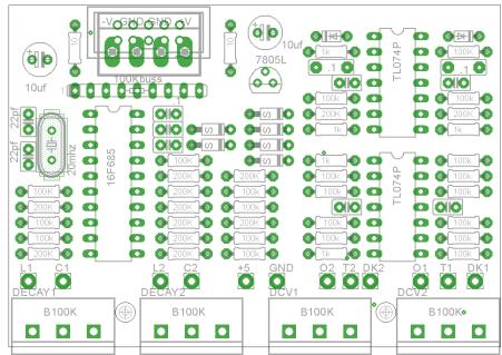
DK1 / DK2 for the CV/Decay input jacks O1 / O2 for the output jacks
