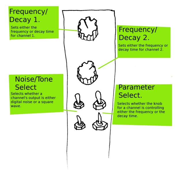
KNOB1, KNOB2 = Sets frequency or decay time based on the parameter select toggle for that switch.
