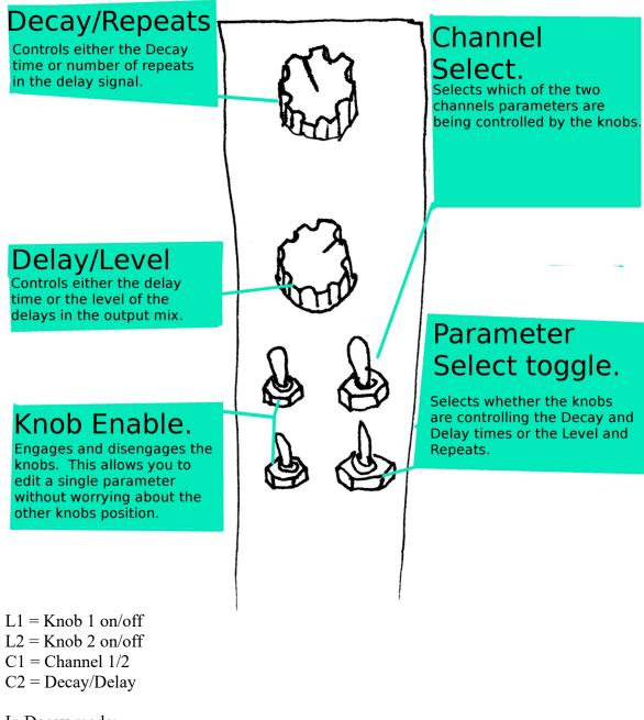
In Decay mode: Knob 1 is Decay Time Knob 2 is Delay Time
