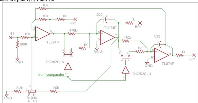
The output of the comparator is then attached to the input pins of the DG202 analog switch, these are pins 1, 8, 9 and 16.
