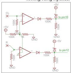
**F.Outputs.** To the right are the outputs. Each is identical, it consists of an op-amp wired as a buffer whose output is going to an indicator LED and an output jack.
