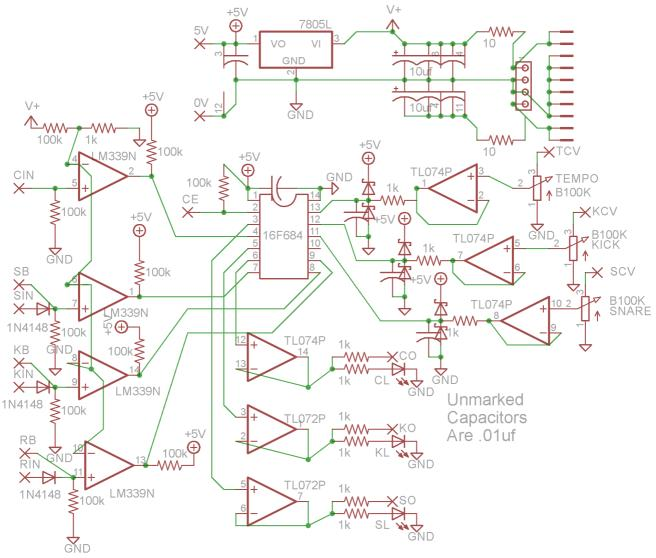
Above is the schematic for this project. The 16F684 is the heart of the module, it processes the input circuitry from the external voltages and gates and creates the triggers. Pin 2 of the PIC has a 100K pull up resistor and is attached to the "CE" or "Clock Enable" wirepad. This wirepad will
