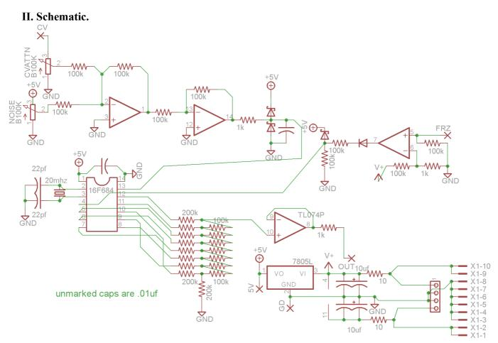
Above is the schematic for this project. The 16F684 is the heart of the module. It's clock is derived from a 20mhz crystal and it's power supply is +5V. I'll describe it's inputs first, then it's output, and finally the power connections. I will use terms without providing a definition, if you'd like to know more about how a comparator or an R/2R works, there are plenty of free online resources that can explain better than I can.
