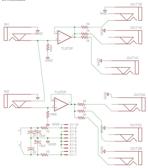
Above is the schematic for this project. The first input jack's tip is connected to the switch of the second input jack so that when nothing is plugged into the second jack the first jack's signal will go to all six outputs.
