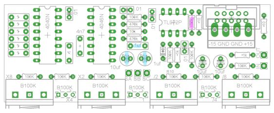
Above is the PCB. Highlighted in purple is the mixing resistor for the output. **IF BUILDING ON A 15V SYSTEM REPLACE THIS WITH A 68K!**
