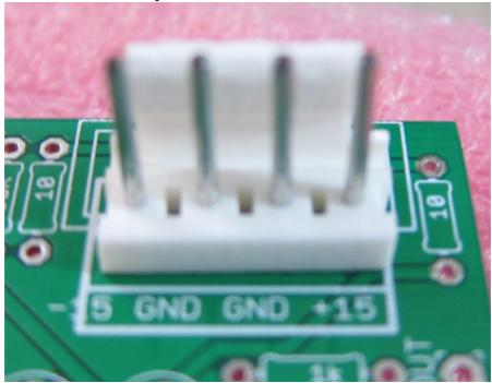
If you are using a Eurorack style connecter, it should be connected as shown on the PCB, with the tab facing out and the red line nearer to the wiring pads.
